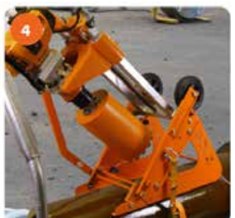
45° Drill in cast iron pipe. Fixing by strap, clamping ratchet and angle support (accessory).
